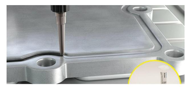
One component epoxy adhesive is widely used in different high-volume assembly line applications, including bonding, encapsulation, sealing, and potting. It is commonly used in the automobile, aerospace, electronic devices, and medical sectors, to name a few, because of its exceptional bond strength, chemical resistance, and sturdiness.
